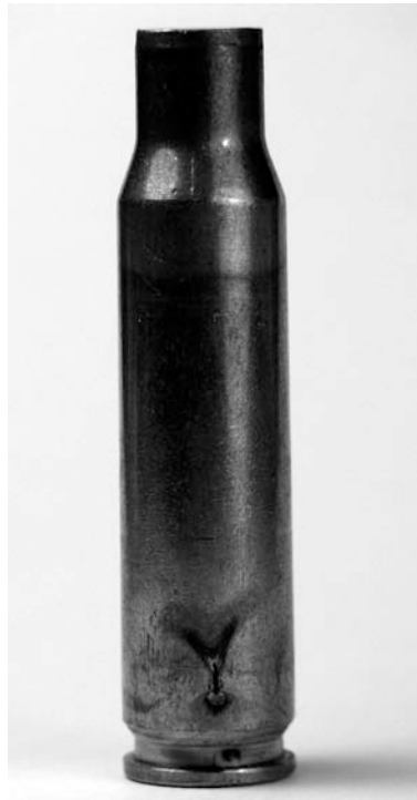
Old factory loaded case with split allowing gas to escape on firing.
